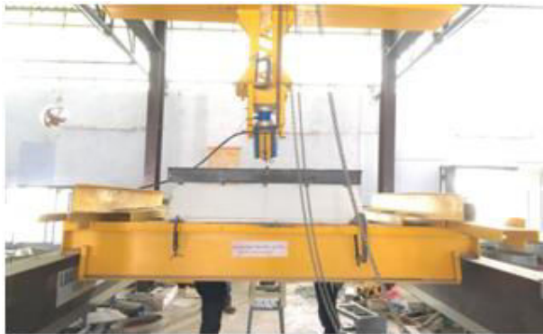
Figure 8: During testing of Ferrocement folded plate
