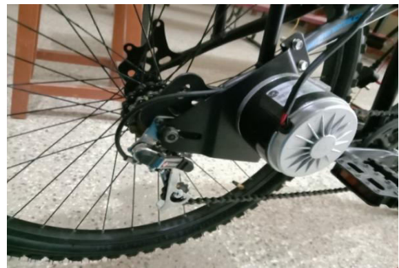
Fig.3.View of PMDC motor mounted to the rear wheel of a bicycle
