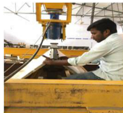
Figure7: placing of specimen on loading frame
